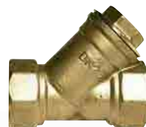
Filtro "Y" tamiz inox MT PN-16 1", 1/2", 3/4". CW617N. Malla inox. 875FY11
